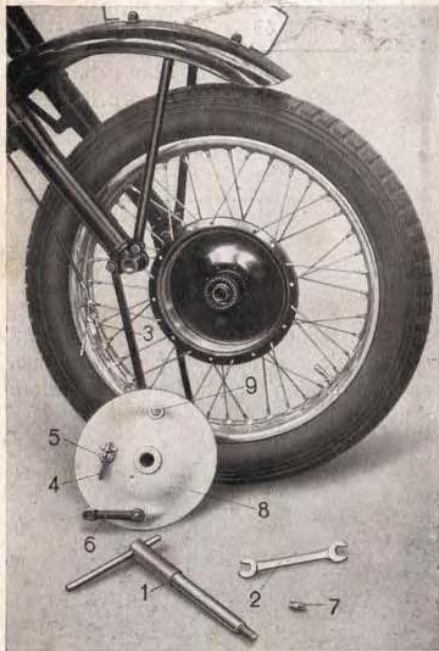
Fig. 1 Disassembly of the front wheel.
